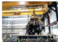
Crane operator feed mixed waste to Waste Hopper
